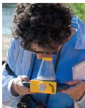
Figure 1.26 A field microscope – this is used to investigate the structure of specimens in the field, whilst still fresh
