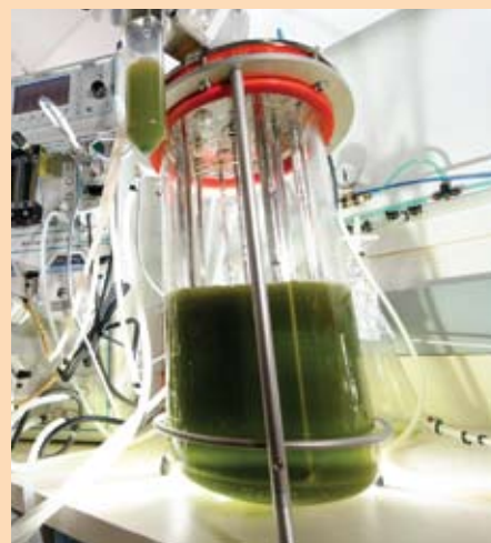
Figure 5.26 A fermenter that monitors changes electronically
