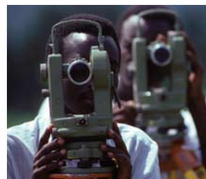
Figure 1.27 A theodolite – this is used to measure the height of trees or of slopes in the area
